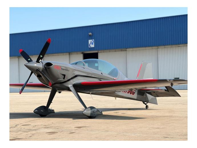
Finished in a striking custom factory paint scheme, this aircraft combines cutting-edge aesthetics with unmatched performance. Powered by the Lycoming AEIO-580-B1A engine and a MTV-14-B-C190-130 four-blade composite propeller, this GB1 delivers top-tier aerobatic performance—perfect for solo routines or sharing the adrenaline with a passenger.
