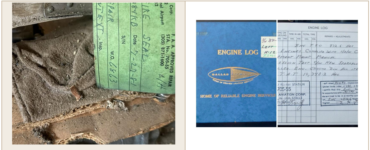
Left: surviving Sekman Aviation repairable component tag visible with the stored engine assembly. Right: current-condition engine detail. The tag is presented as component-level provenance, not as a statement of whole-engine airworthiness.
