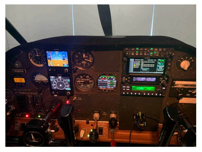
TTAF-2825hrs, Eng-78hrs since Factory Reman, Prop 510hrs since overhaul, factory oxygen, Century III Autopilot with G/S coupler
