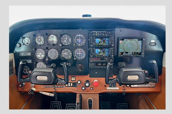
Upgraded Garmin Avionics with Dual Garmin GNS-430W WAAS Nav Comms, Garmin GTX-345 ADS-B In/Out Transponder, & Garmin GMX-200 Multi-Function Display (MFD)
