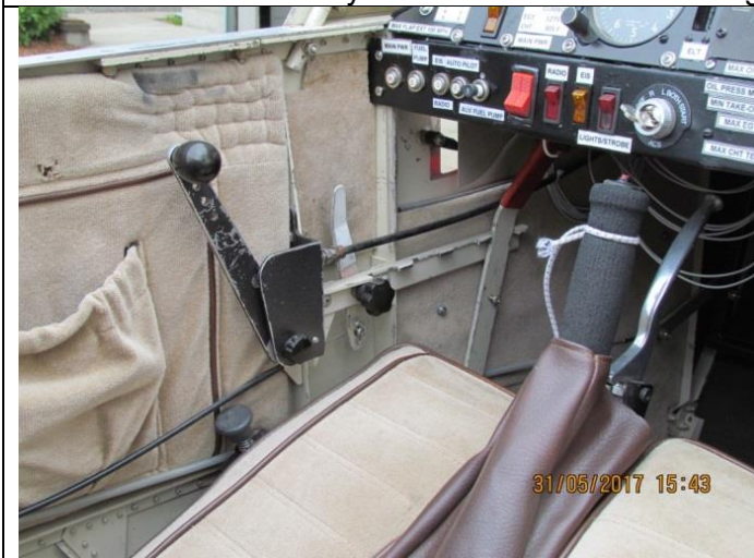
Throttle, flap handle and pitch trim.
