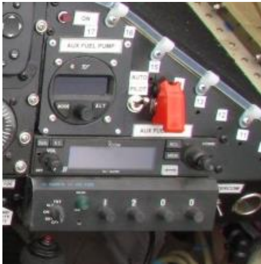
Narco IC-A210 radio, Narco AT 150 TSO Transponder, TruTrak DigiFlight II Autopilot
