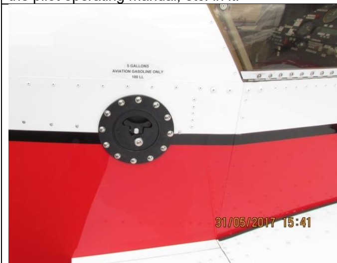
Outside auxiliary tank fill.
