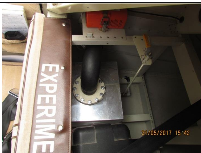
Five gal. auxiliary fuel tank with shut-off valve
