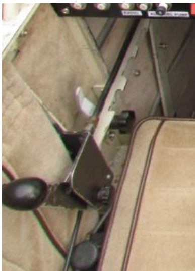
Side mounted throttle, three position flap handle and elevator trim lever
