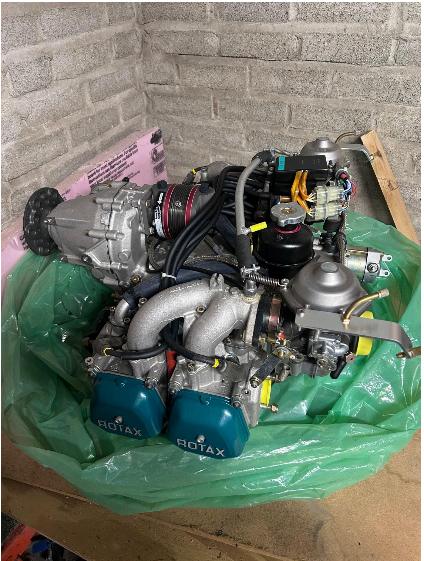
Rotax 912ULS 100 hp Engine with Vacuum Pump. Will need the 5 year rubber replacement and recommend carb overhaul.
