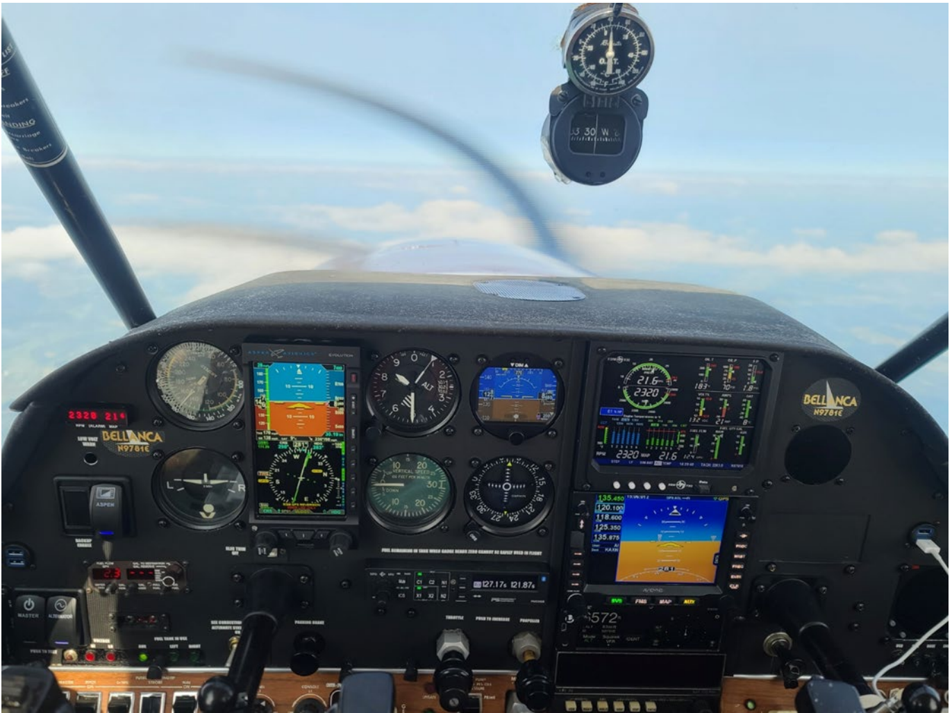
Current panel in-flight (autopilot removed)
