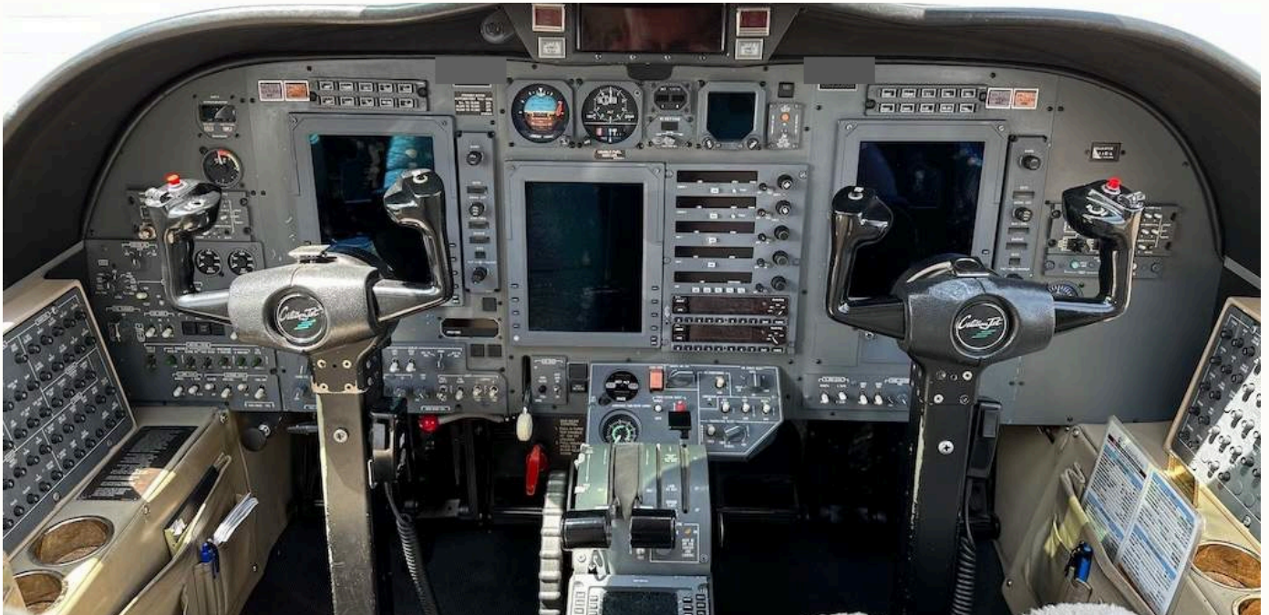
COLLINS PRO LINE 21 FLIGHT DECK · DUAL AHRS · UNIVERSAL UNS-1K FMS
