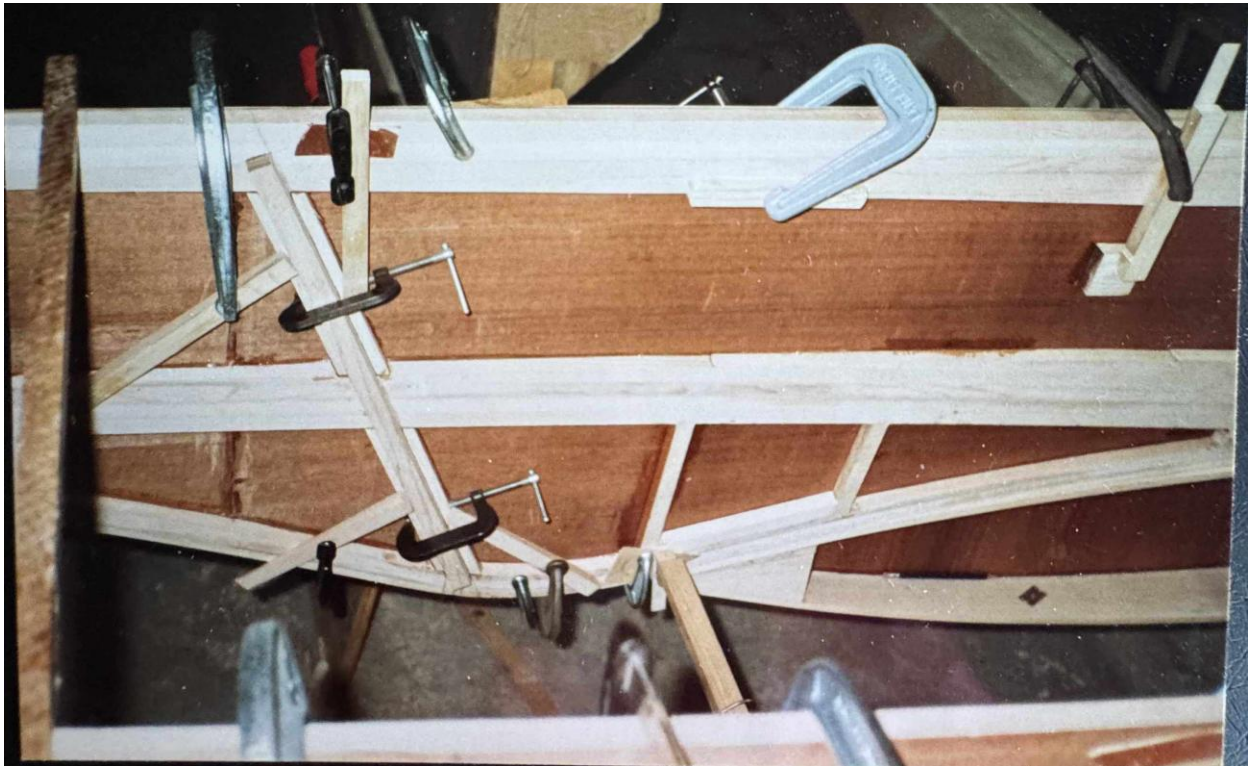
Port fuselage side-view at wing trailing edge before inner skin attachment
