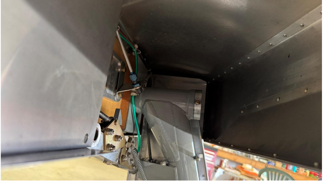
Port wheel well upper main gear and trunnion assembly
