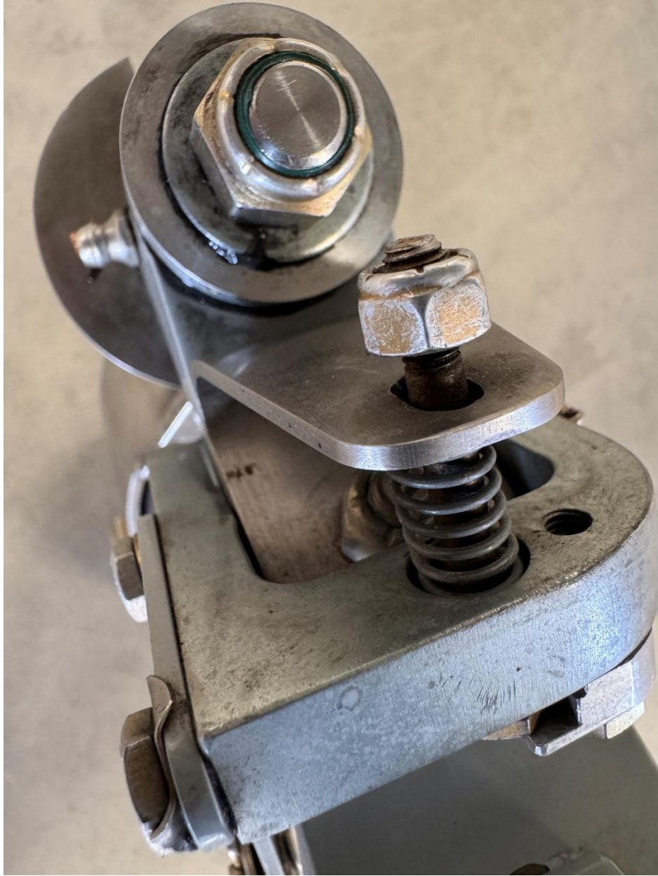
Tailwheel mechanism, view top-down
