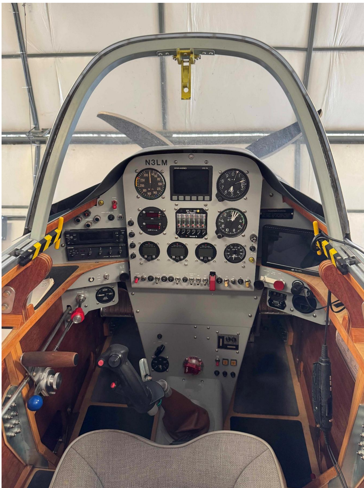
Front cockpit yellow and black canopy emergency release. Center lower panel fuel management controls. iFly EFB GPS side panel.
