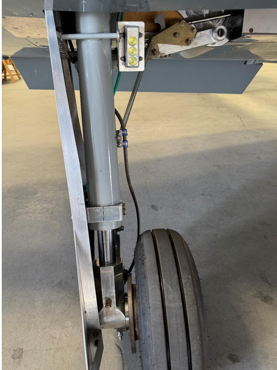
Main gear down and locked; Taxi light shown
