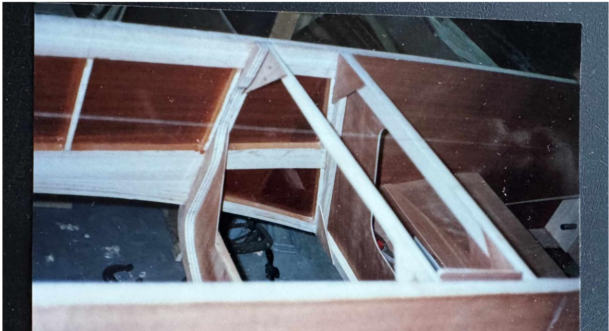
Port fuselage side-view aft of rear seat back before inner skin attachment
