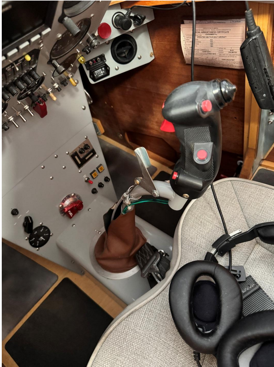
Pistol grip control stick with shiny tail wheel unlock lever
