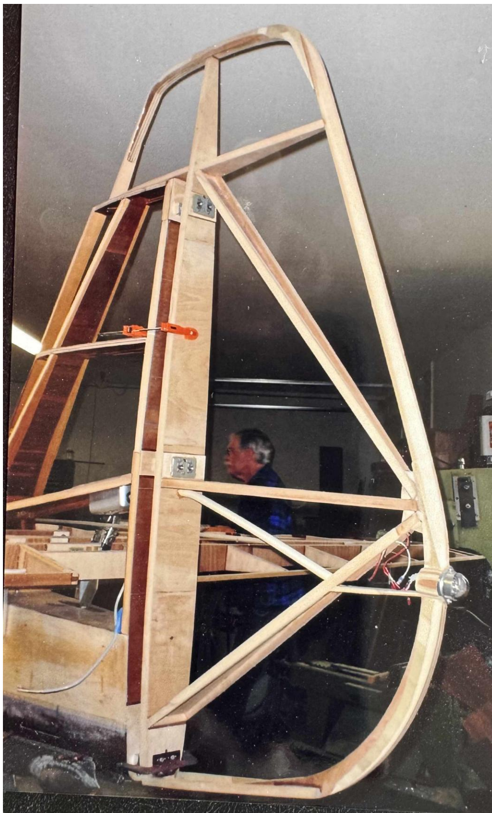
Rudder structure hinge fitted
