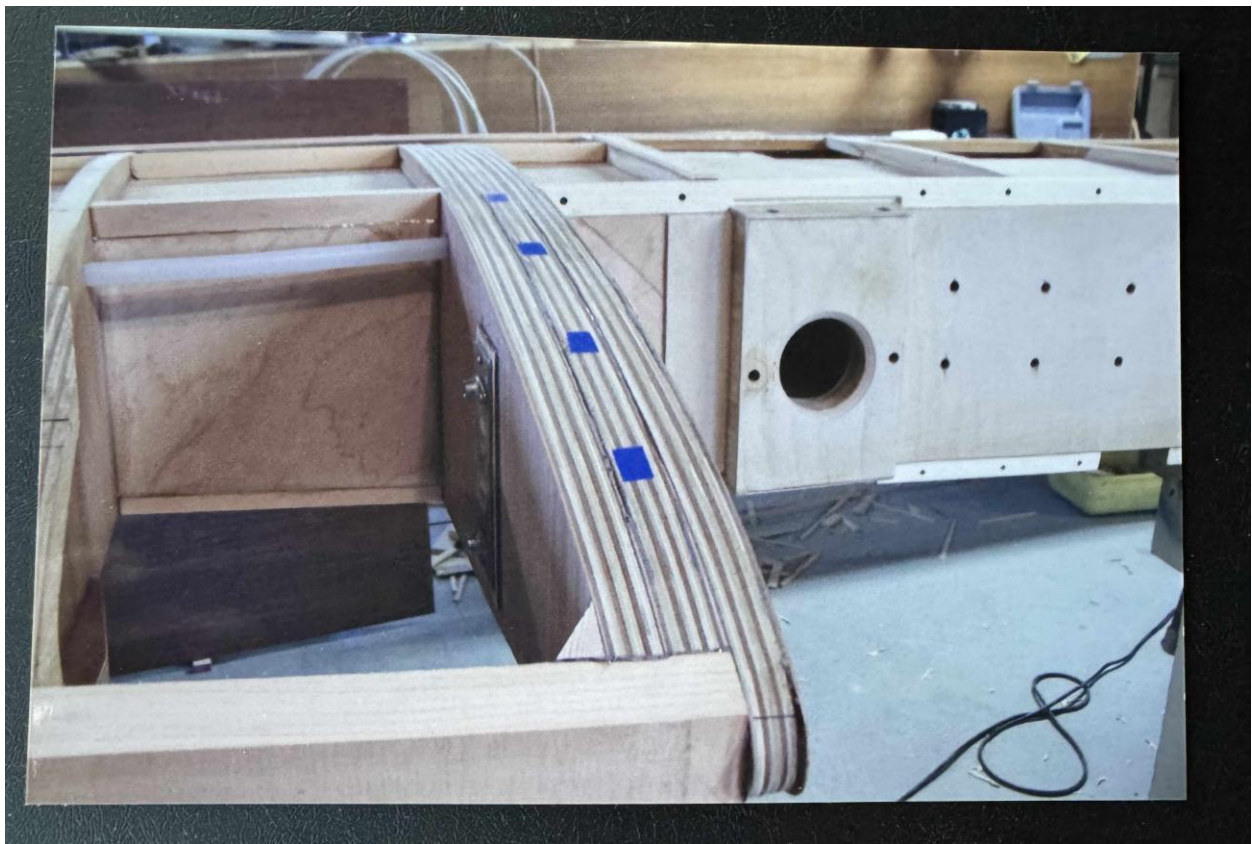
Rib number 4 and landing gear trunnion hard point
