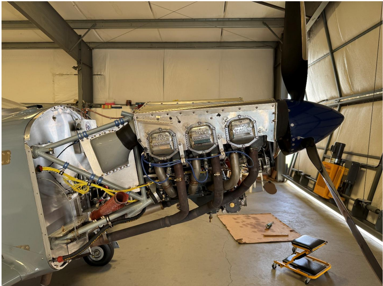
Starboard view: Plenum and titanium firewall
