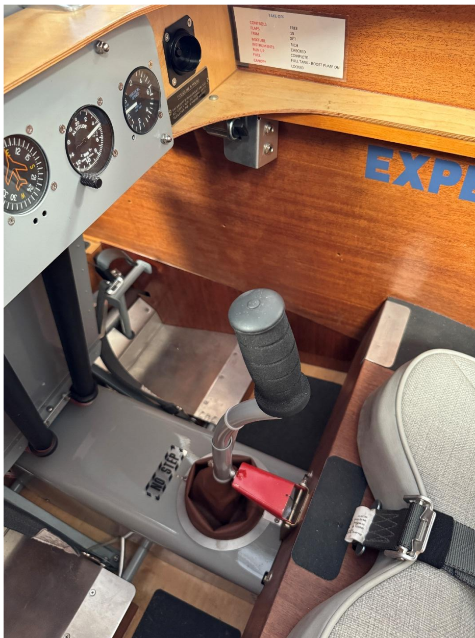
Rear control stick with red control lock engaged
