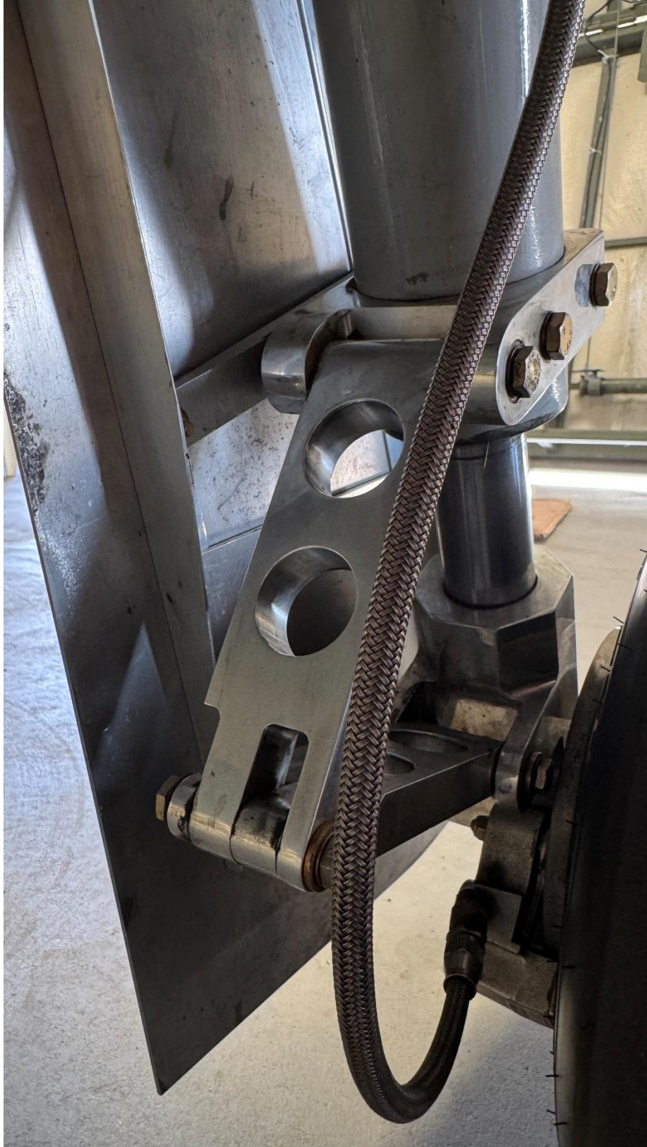
Port landing gear scissors
