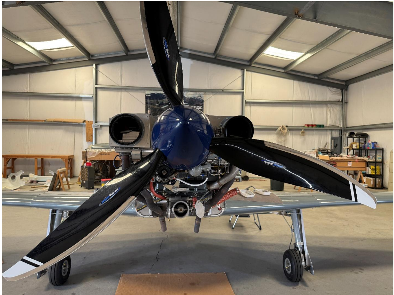
Plenum inlets and tuned cold air induction
