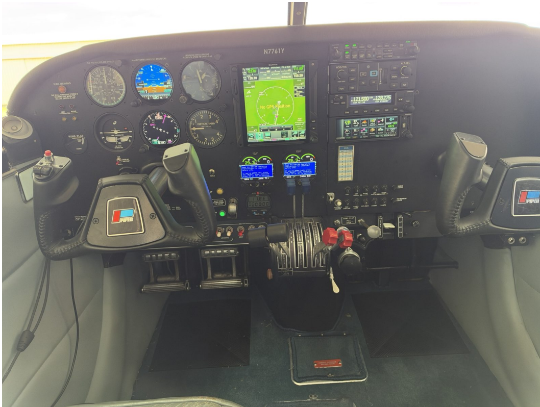
Panel: GTN 750Xi, GNX 375, GTR 225, GFC 500, GMA 345, dual GI 275, dual CGR-30P
