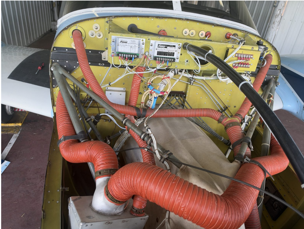
Nose bay: dual Plane Power voltage regulators and clean wiring (current photo, 10/2026)
