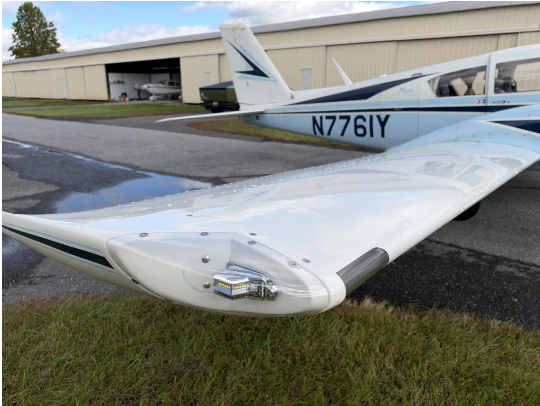
Johnston wingtip with Whelen Orion LED nav/strobe
