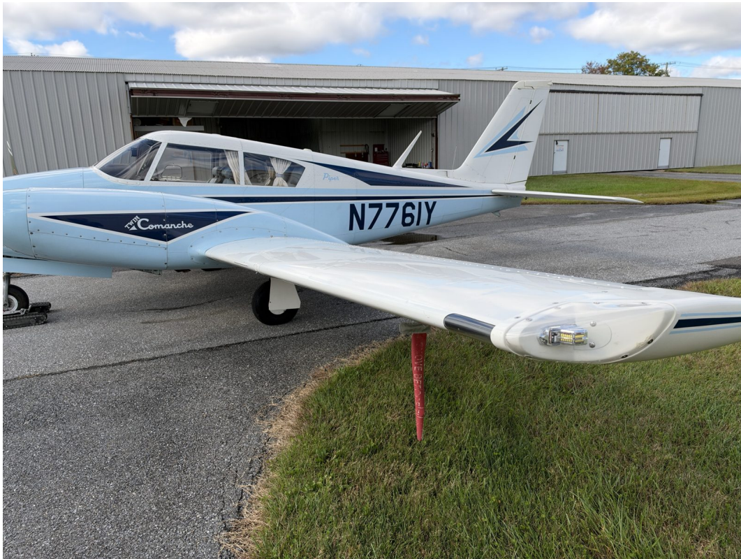
Left side, with Whelen Orion LED wingtip lights
