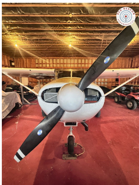
Front view, McCauley two-blade constant speed propeller.
